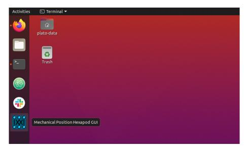
A desktop entry is defined in a file with the .desktop extension. The content of the desktop file for the Mechanical Position Hexapod is shown below. The desktop files for several Task GUIs are located in the repo folder ~/git/plato-common-egse/client/.
